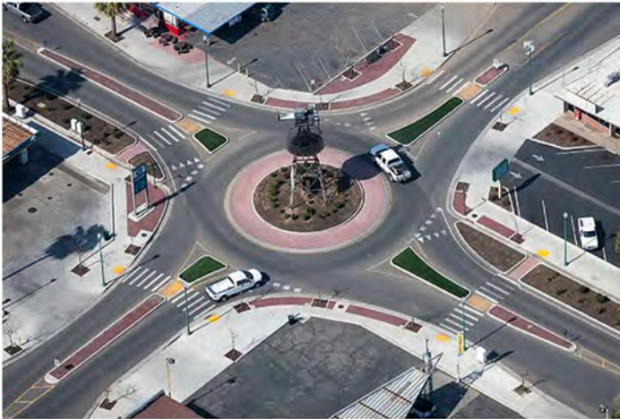
Figure 3.9.1. Single-Lane Roundabout (Source: Omni-Means, Ltd.)
